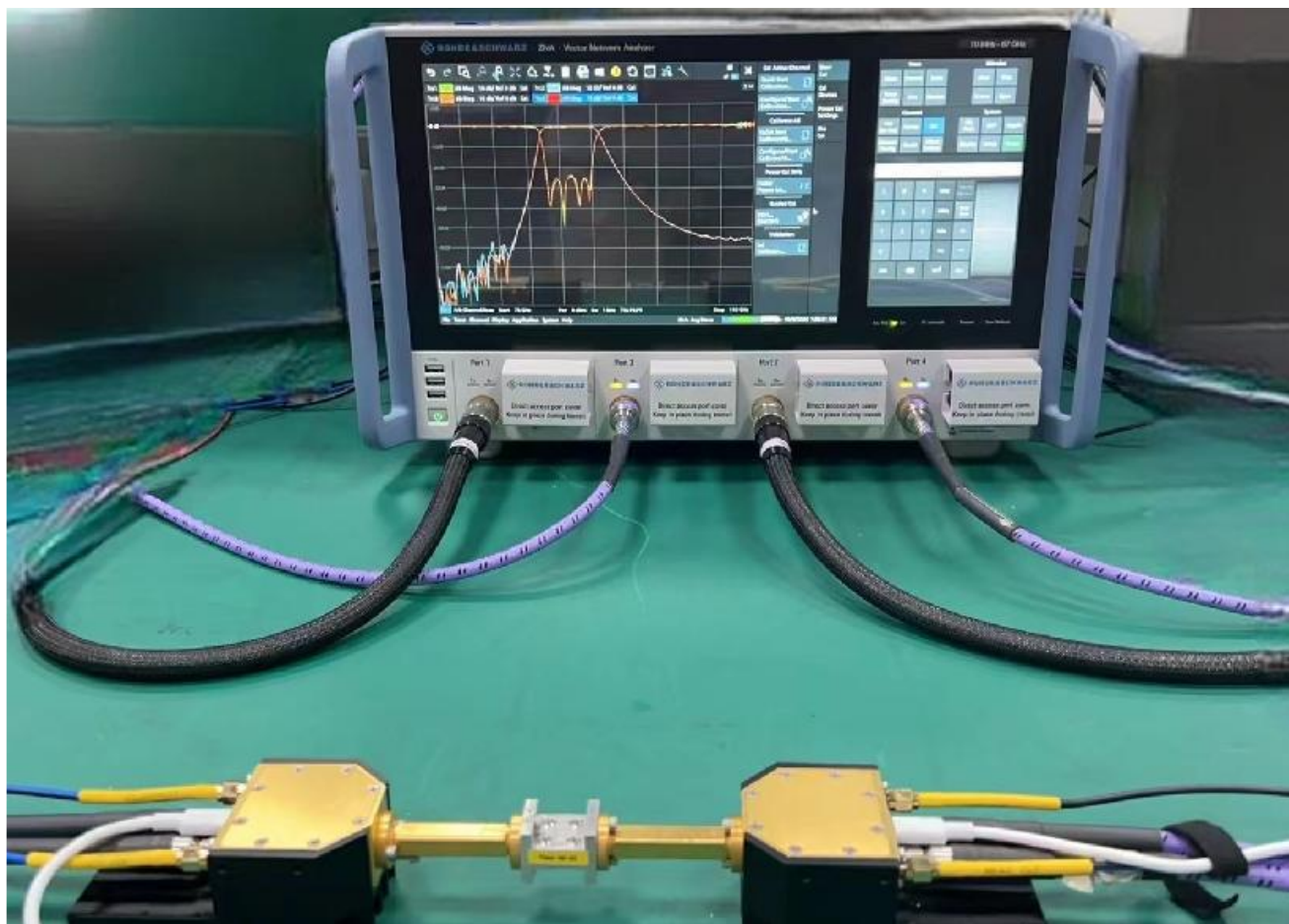
QS-1000TRs connection test with R&S VNA
