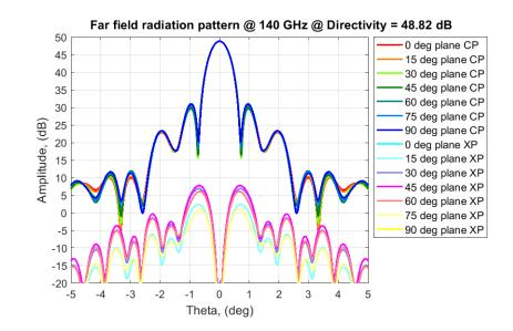
\* Radiation Pattern of CRS-240-WR06. Contact us for the performance of any model.
